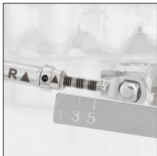
Laser Marked Visual Indicator on Arm and Splint for Advancement Confirmation
